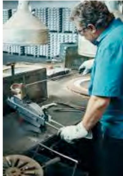
Door handles in aluminium are cast by hand. The lightweight metal is scooped out at a temperature of 660 degrees Centigrade and formed into the required shape by a process known as gravity die casting: the aluminium fills the shaped cavity with the aid of nothing but the force of gravity.
